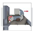
Advanced cam design rotates hook away from RIG first to release pressure from RIG Wedge.
