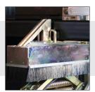
Push-button operation to raise the restraint and engage the Rear Impact Guard.
