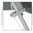
Float barrel hold down is designed to operate under extreme float conditions common with air ride suspension trailers.
